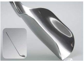
PharmaSpoon for taking samples of powdery substances, intermediate products and material in the pharmaceutical industry. Special materials with excellent surface qualities must be used for this to prevent cross-contamination. Our PharmaSpoon fulfils these requirements. Made of stainless steel AISI 316L (1.4404), surface highly polished by hand (not electro-polished!). The excellent surface properties of the PharmaSpoon provide significant advantages.
