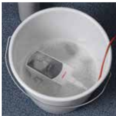
TF 410 - still working, thanks to IP67
