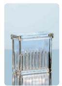
For 16 microscope slides 76 x 26 mm, with widening towards the top. Note: Do not clean staining dishes and staining jars at temperatures above 60  $^{\circ}$ C (glass corrosion is possible).
