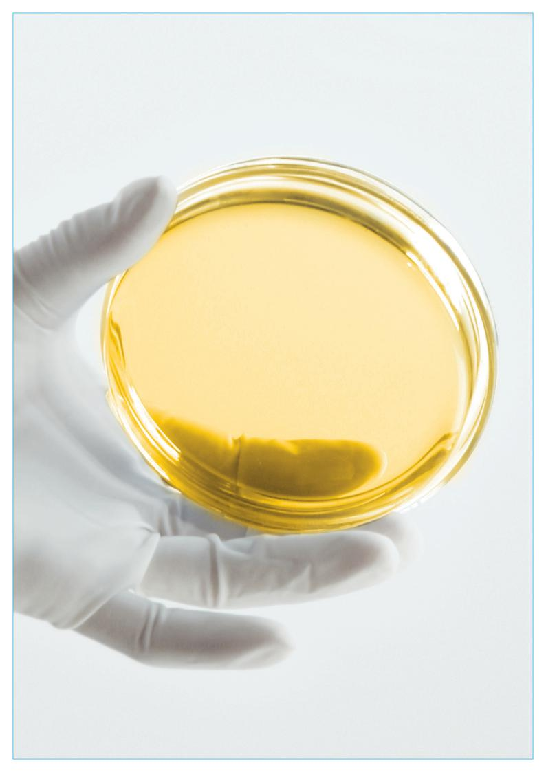
Due to its high thermal-shock resistance, DURAN® microbiology glassware is ideal for auto-claving and sterilisation processes and shows, even after multiple use no signs of wear. Unlike plastic items, it is very resistant to mechanical wear even after repeated use and sterilisation cycles.
